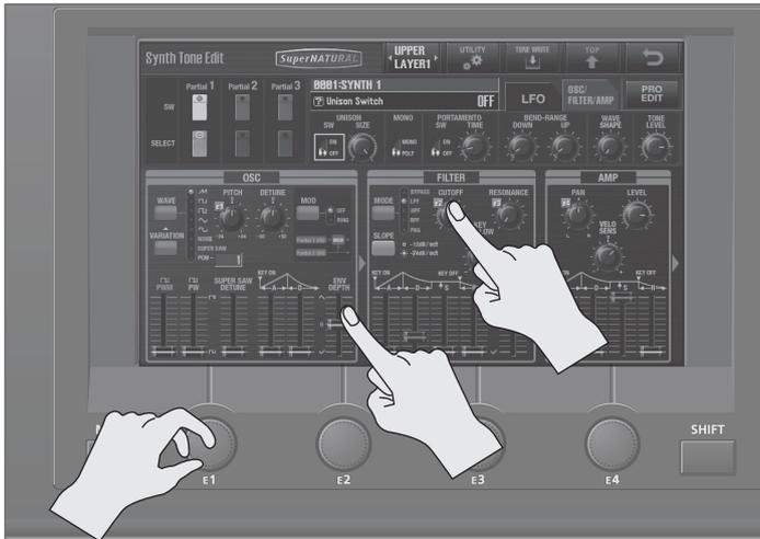
The parameters assigned to the [E1]–[E4] knobs are indicated by icons E1–E4.
