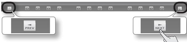
Pressing the [NEXT] button switches to the next Registration Set; pressing the [PREV] button switches to the previous Registration Set.
